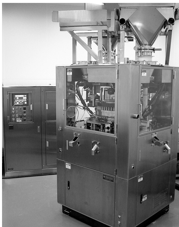
Fig. 4 Newly-developed rotary tableting machine for OSDRC (PAVO 0554SW7KZ).
