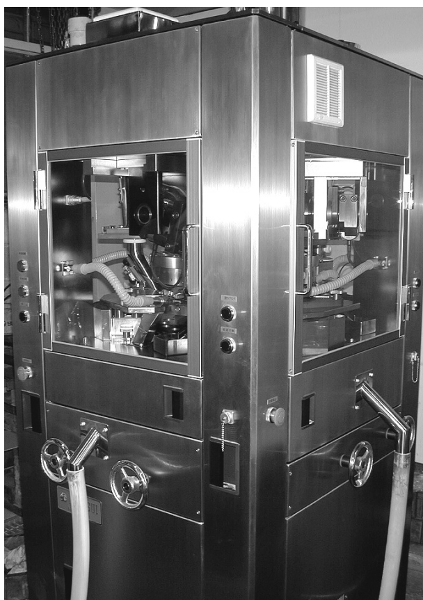
Fig. 3 Rotary tableting machine for OSDRC (PAVO 0521SR).
